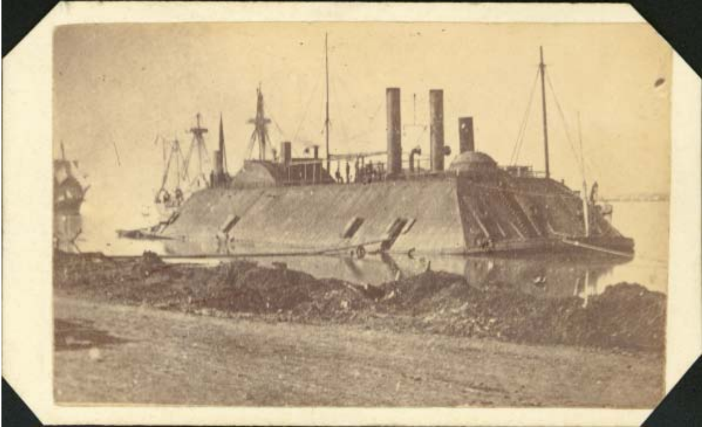
U.S.S. Essex off Baton Rouge. The U.S.S. Essex was converted in stages from the steam ferry "New Era" into a 1000-ton ironclad river gunboat. Essex's Commanding Officer, William D. Porter, spared little expense in upgrading his ship into one of the most powerful ironclads on the Western Rivers. After joining Rear Admiral Farragut's squadron as the only Federal ironclad on the lower Mississippi, she helped repel an attack on Baton Rouge, Louisiana, on 5 August 1862 and was instrumental in the destruction of the CSS Arkansas the next day. Marshall Dunham Photographic Album (Mss. 32410109), Louisiana and Lower Mississippi Valley Collections, LSU Libraries, Baton Rouge, Louisiana, USA. Mark Martin's remarks about this amazing album begin on p. 17.
